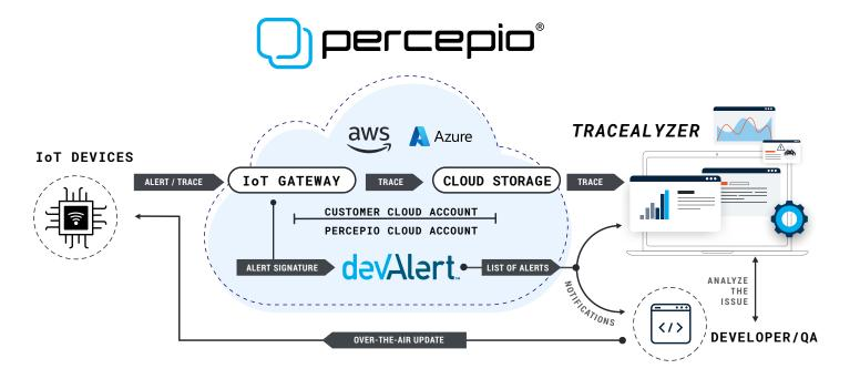
Alerts may also include a trace of the most recent software events in the device, recorded automatically by the agent. The trace provides details of the error and the context, making it easier for developers to identify the bug.
