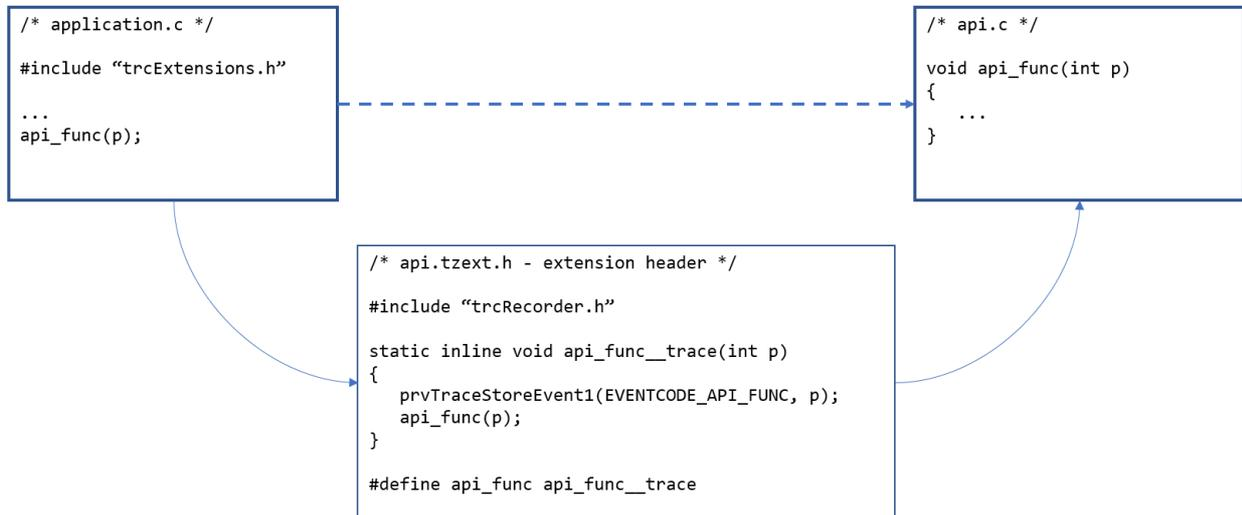
This works for regular function calls and also for function pointers/callbacks, since the initialization of the function pointer is also affected by the redefinition. And since the traced function is not modified, this even works with binary libraries and assembly functions.
