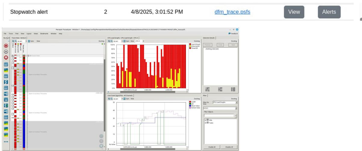
This will open the trace in the Tracealyzer tool, included in the Detect Client. The trace data comes from the TraceRecorder library, that supports both RTOS kernel tracing and several kinds of application logging. The tracing is based on kernel instrumentation and logging calls. The events are written to a circular RAM buffer. On alerts, the trace buffer is included as a payload and shows the most recent events before the alert. Tracealyzer traces can be included with all alert types.
