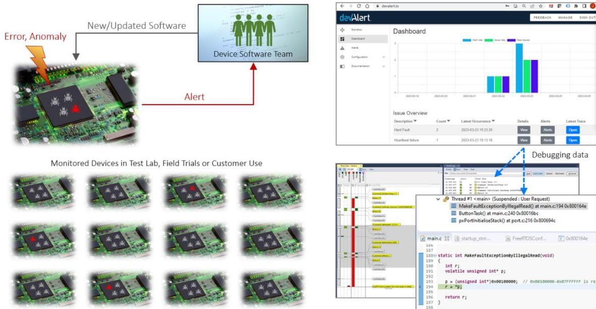
DevAlert gives your team members a shared dashboard with remote access to diagnostic data, automatically collected in the devices on system errors and other anomalies. This may include core dumps, event traces and any other device data of interest.
