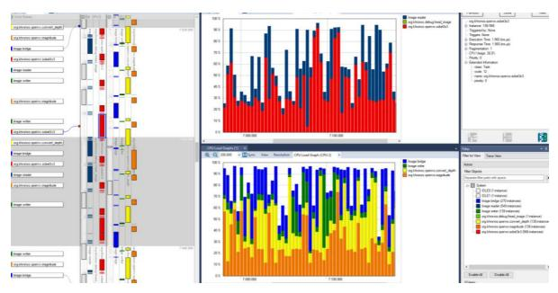
All views in Tracealyzer are interconnected in similar ways, which makes it easy to drill down from high-level overviews into the detailed trace. The colors are used to make it easier to identify the OpenVX graph nodes. The same color coding is used across all Tracealyzer views.
