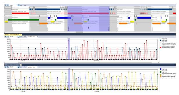
The Actor Instance Graph can show various timing properties, not just execution time, but also e.g. separation and periodicity. You can change what property that is displayed in the dropdown menu that reads "Execution Time" by default. Some of the properties are however not very relevant for OpenVX traces. For instance, Response Time will always be equal to the Execution Time due to the run-to-completion scheduling.
