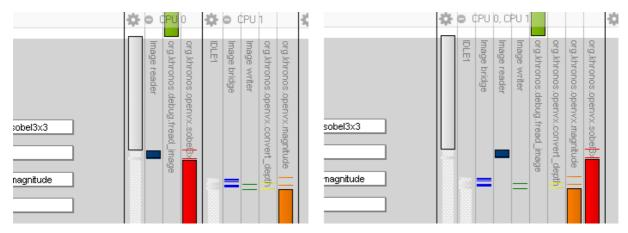
The Trace View is composed of fields, above labeled "CPU 0", "CPU 1" in the left example. There are several types of fields for different types of information. OpenVX nodes are shown in a "scheduling" field, either one field per CPU core (left example) or a single field for all nodes (right example).
