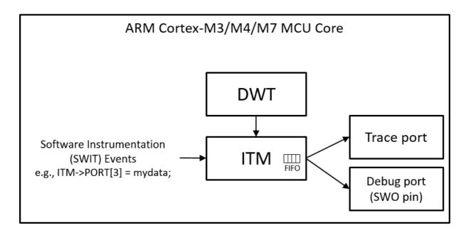
With a fast debug probe ITM allows for high data rates (over 2 MB/s) and the target-side overhead is minimal. In our experiments, writing 16 bytes of data took just 55-60 clock cycles, despite requiring four separate writes. Moreover, unlike some other streaming solutions we support, ITM tracing does not require any RAM buffer.
