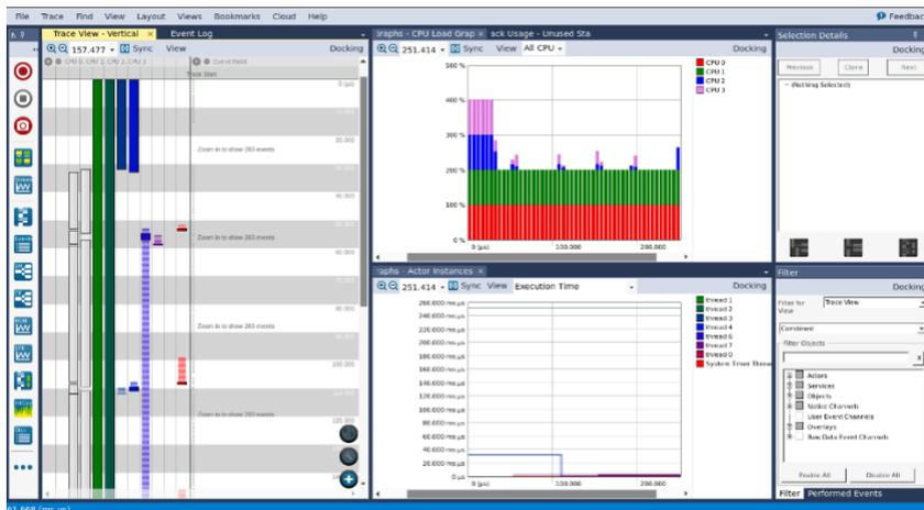
Tracealyzer showing Azure RTOS ThreadX SMP running on four cores.
