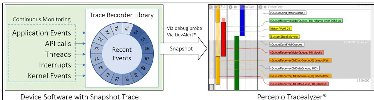
Snapshot tracing is now available for Zephyr RTOS. This allows for tracing without special hardware and can even be deployed in production devices.
