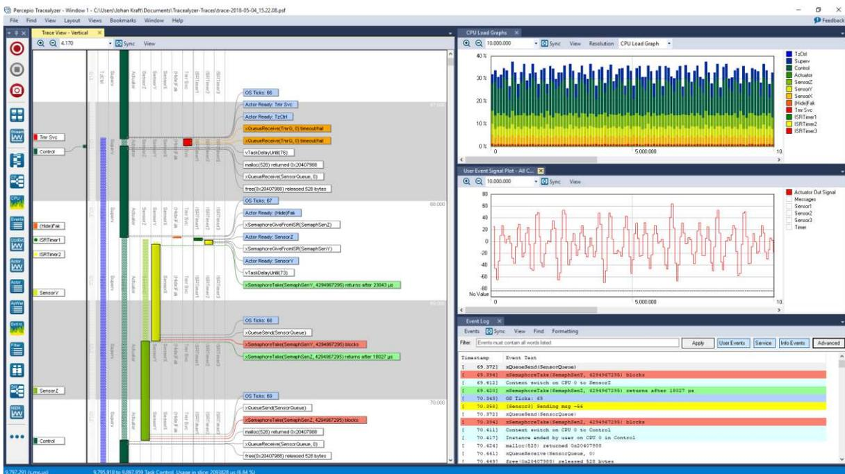
As of version 4.1, Tracealyzer supports [ITM tracing](#) for ARM Cortex-M3, M4 and M7 MCUs. This is initially available for FreeRTOS and Micrium  $\mu$ C/OS-III, but support is planned for SafeRTOS and ThreadX soon. An example screenshot of Tracealyzer using this setup is shown above.
