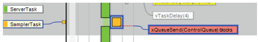
Figure 2. SamplerTask blocks on a send-to-queue operation.
