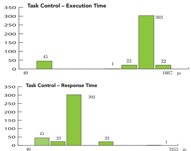
Figure 3. Distribution of execution times and response times (in \mu s) for the task instances.
